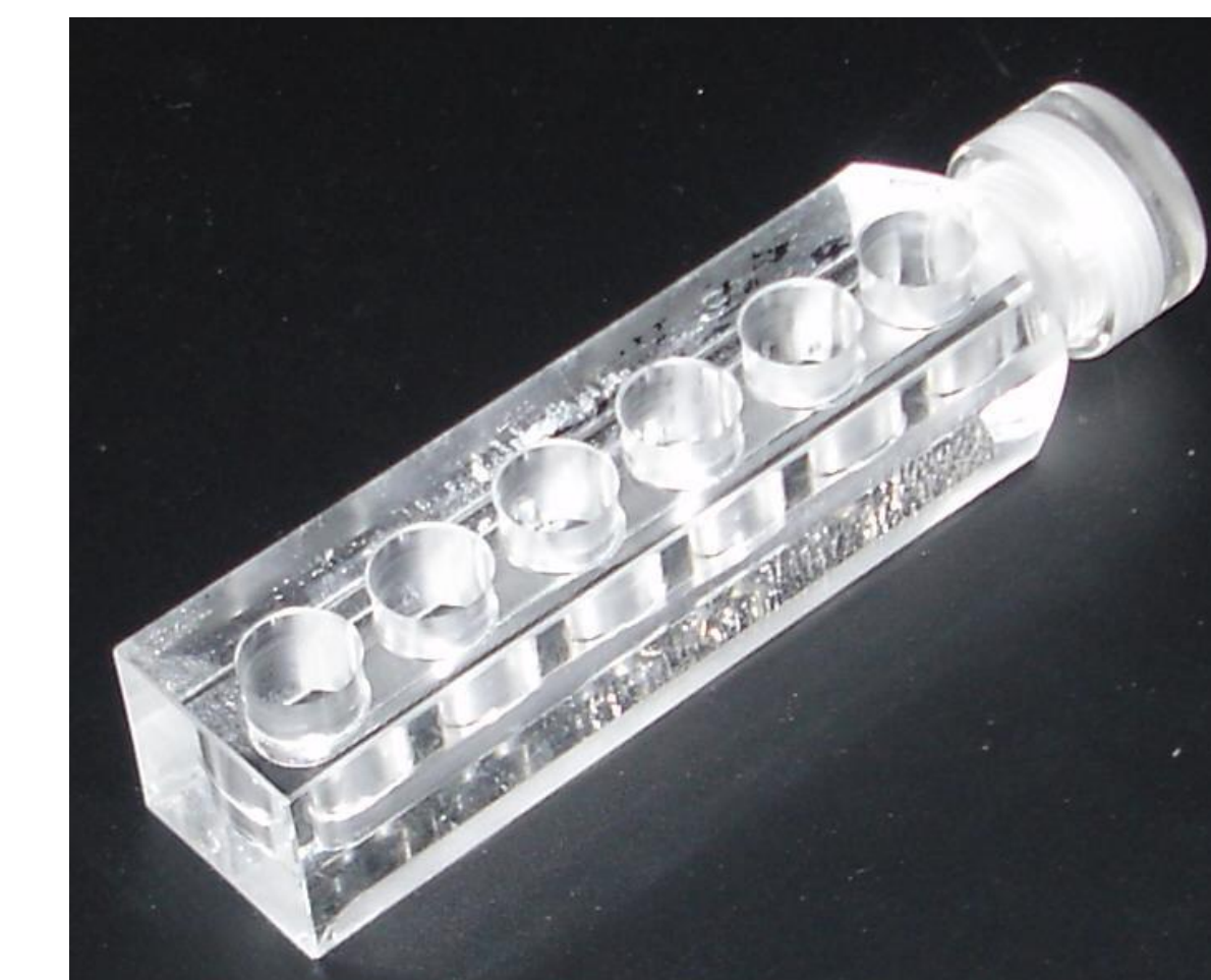
Figure 4. Static Testing Device. This static testing device allows for up to 6 sampling plugs to be immersed in a liquid medium.
